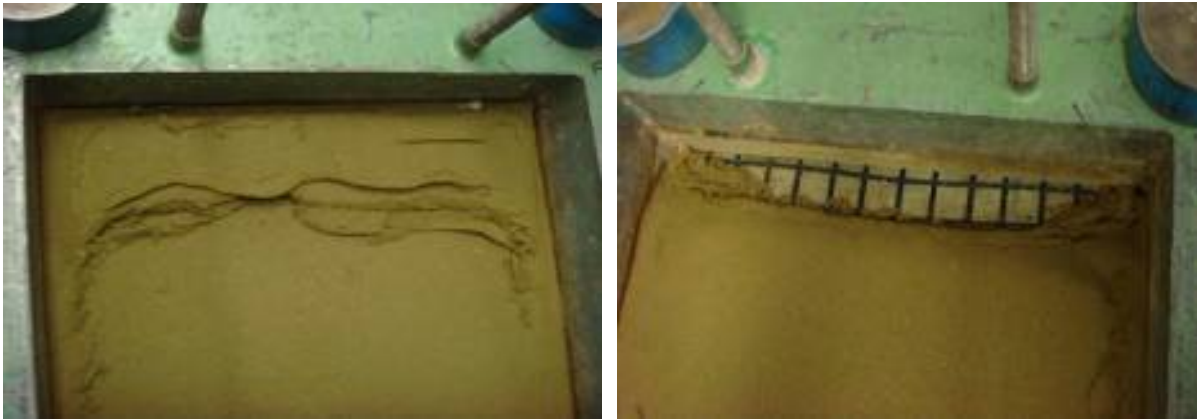
Figure 2. Test on geogrid with soil (a) front side (b) back side (Test 3)
