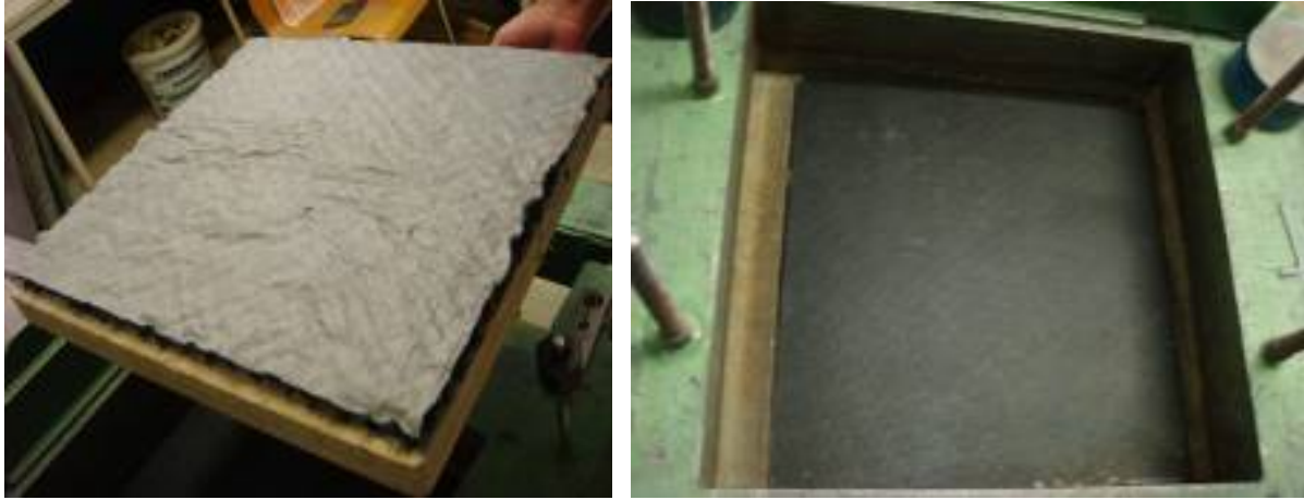
Figure 1. Geocomposite and geomembrane after testing (Test 1)
